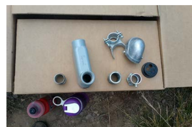
Conduit connection including metal and rubber components of weatherheads, to keep moisture out of conduit.
