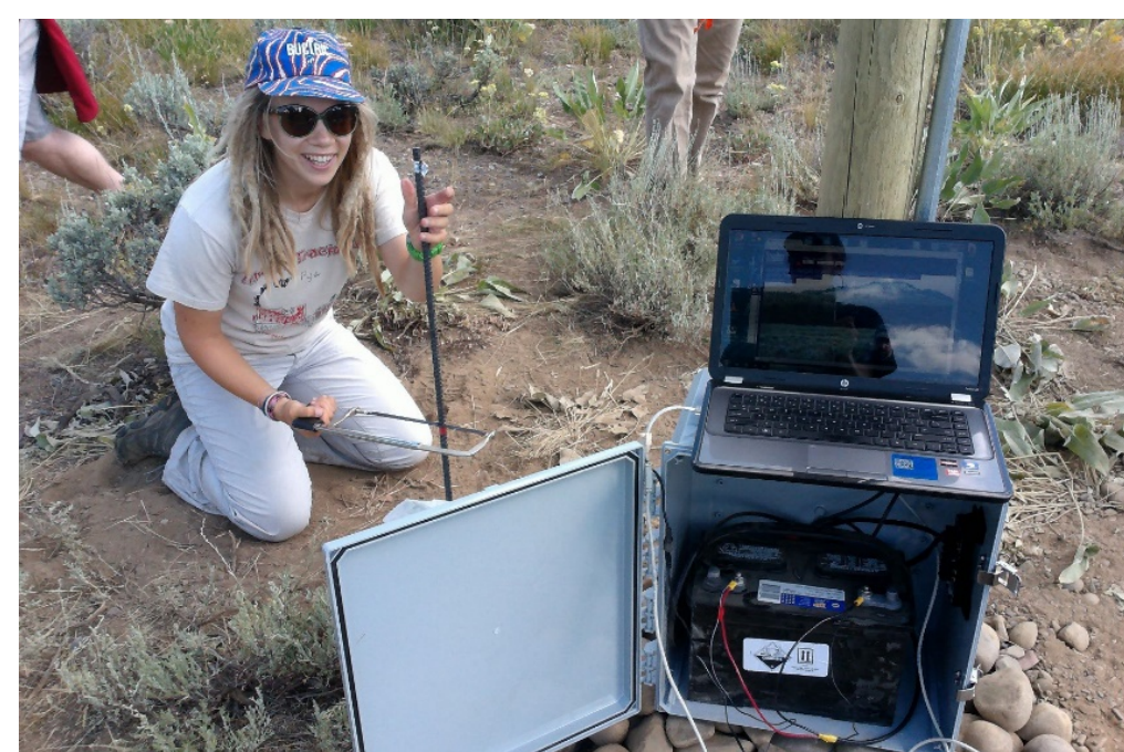
Toni shortening grounding rebar after it was pounded into the ground. Also shown is battery inside Mier box.
