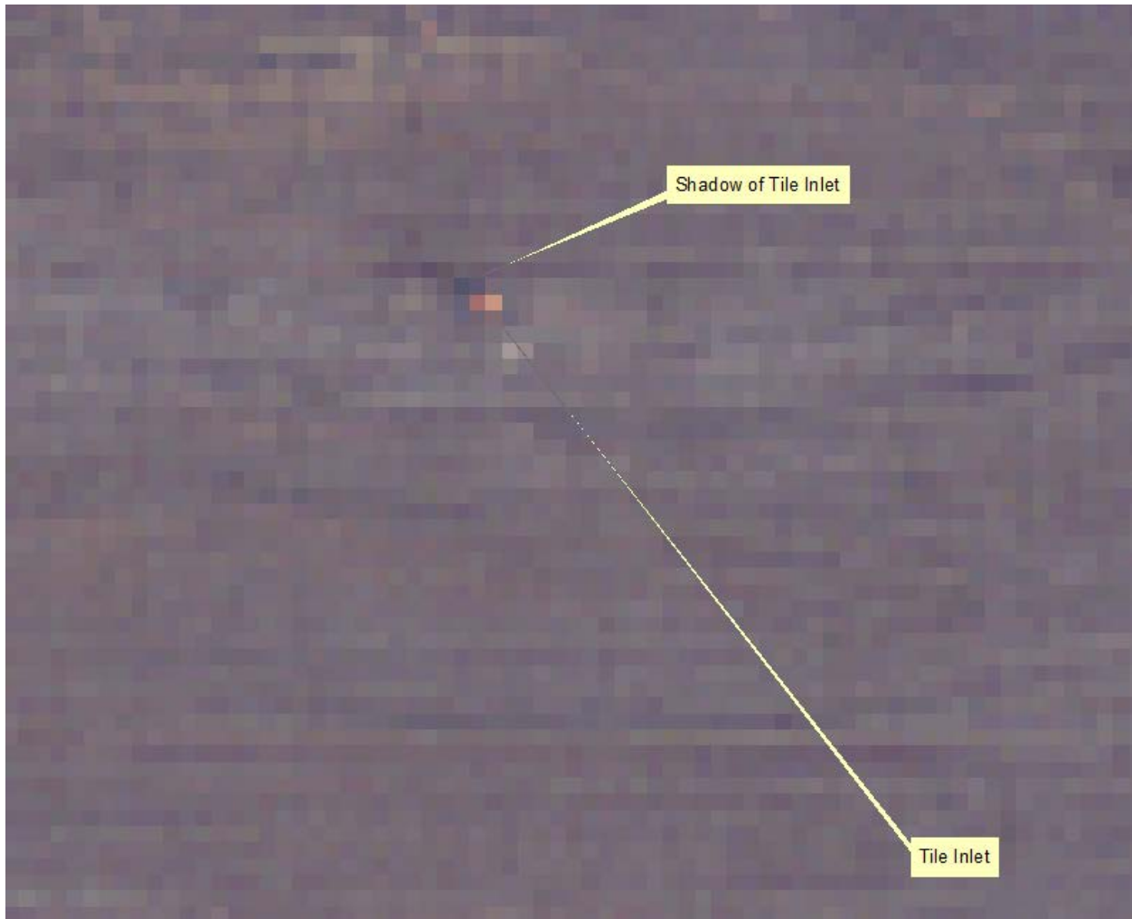
Figure 16C: Close up of the tile inlet in Figures 16A and B. Notice the red-orange color in this Ortho2013 Natural Color image and the dark shadow behind and to the left of the two red/orange pixels. The resolution of the orthophoto is 1-foot, which seems to be the minimum for these features to show up. They blend in on lower resolution images like 1-meter NAIP photos.
