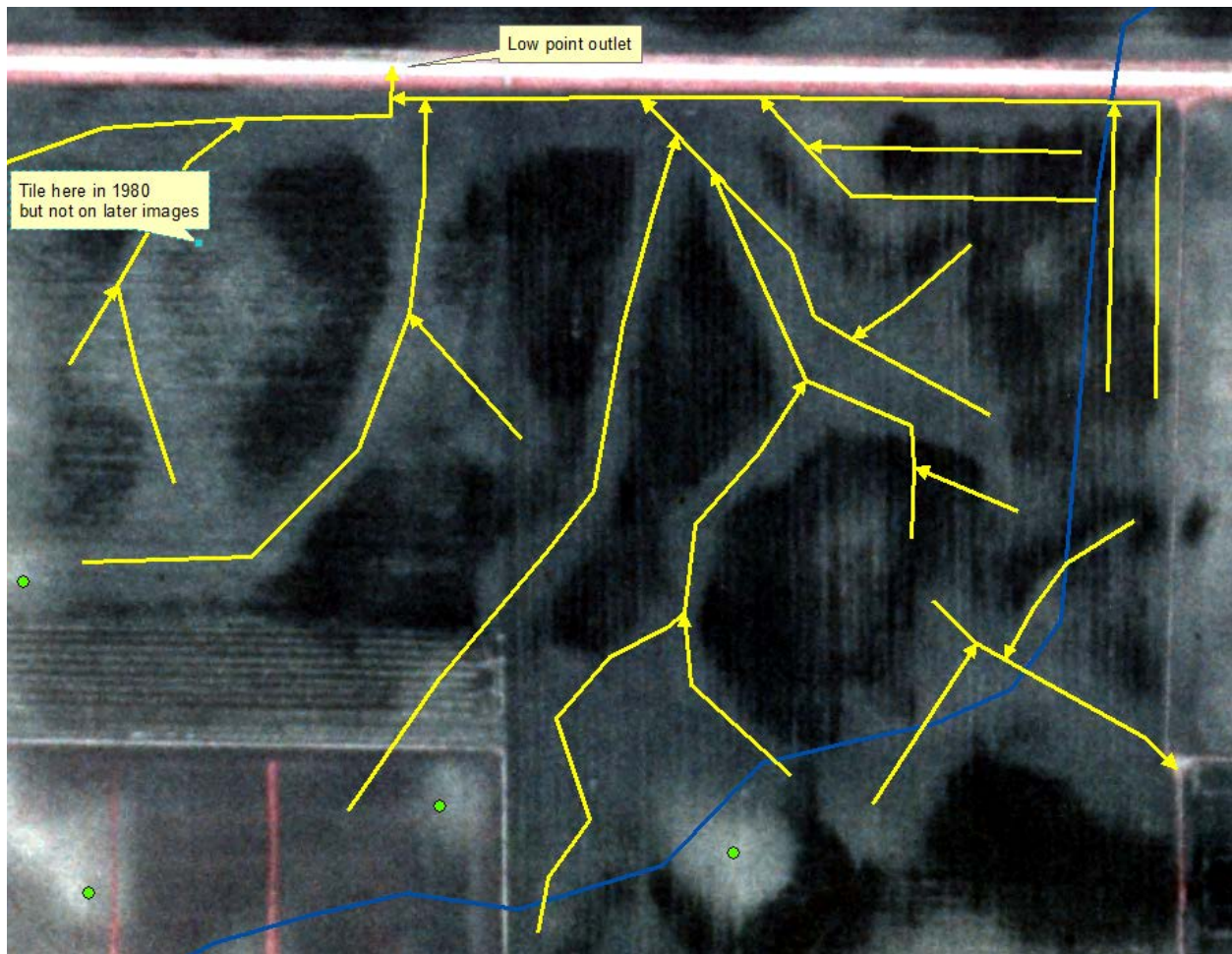
Figure 8: Digitized tile lines using ortho_1980 CIR to find older, irregular tile lines. Notice area on left with lighter tone, a possible tile line, but it does not show up on later imagery, either the 2007 or 2013.
